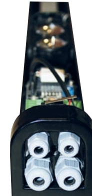
NEW ENCLOSURE WITH CABLE GLANDS
